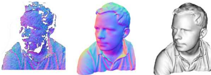
Figure 13.13 Fusing multiple color depth images using the KinectFusion real-time system (Newcombe, Izadi et al. 2011) © 2011 ACM: (a) photograph of the original statue after spray painting with matte gray; (b) partial range scan; (c) merged range scans; (d) colored rendering of the reconstructed model; (e) hardcopy of the model constructed using stereolithography.
