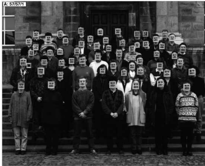
Figure 6.20 Face detection results produced by Rowley, Baluja, and Kanade (1998) © 1998 IEEE. Can you find the one false positive (a box around a non-face) among the 57 true positive results?
