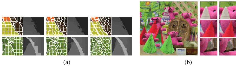
Figure 12.15 Stereo matching with adaptive over-segmentation and matting (Taguchi, Wilburn, and Zitnick 2008) © 2008 IEEE: (a) segment boundaries are refined during the optimization, leading to more accurate results (e.g., the thin green leaf in the bottom row); (b) alpha mattes are extracted at segment boundaries, which leads to visually better compositing results (middle column).
