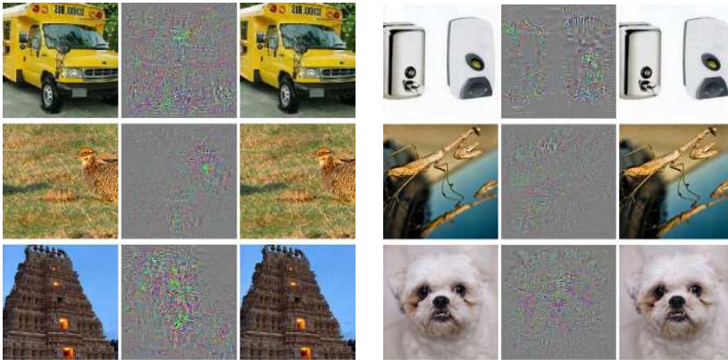
Figure 5.50 Examples of adversarial images from © (Szegedy, Zaremba et al. 2013). For each original image in the left column, a small random perturbation (shown magnified by 10\times in the middle column) is added to obtain the image in the right column, which is always classified as an ostrich.
