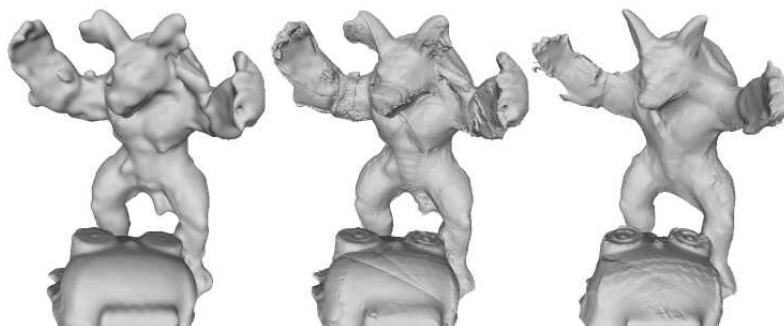
Figure 13.3 Multi-view photometric stereo (Logothetis, Mecca, and Cipolla 2019) © 2019 IEEE: initial COLMAP multi-view stereo reconstruction; refined with (Park, Sinha et al. 2017); and (Logothetis, Mecca, and Cipolla 2019).
