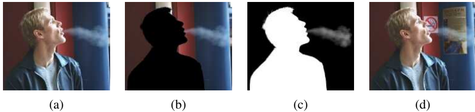
Figure 10.48 Smoke matting (Chuang, Agarwala et al. 2002) © 2002 ACM: (a) input video frame; (b) after removing the foreground object; (c) estimated alpha matte; (d) insertion of new objects into the background.
