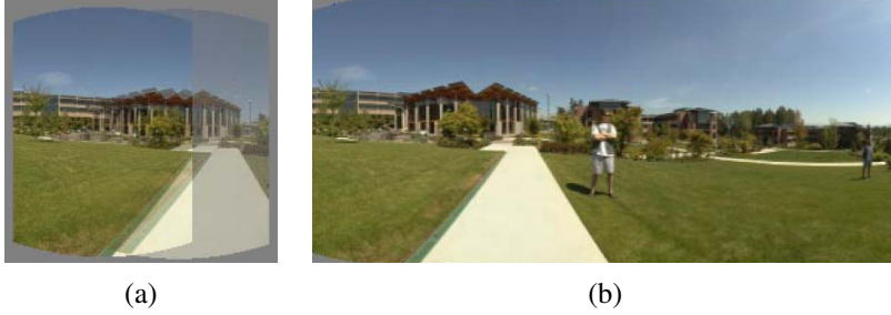
Figure 8.9 A cylindrical panorama (Szeliski and Shum 1997) © 1997 ACM: (a) two cylindrically warped images related by a horizontal translation; (b) part of a cylindrical panorama composited from a sequence of images.
