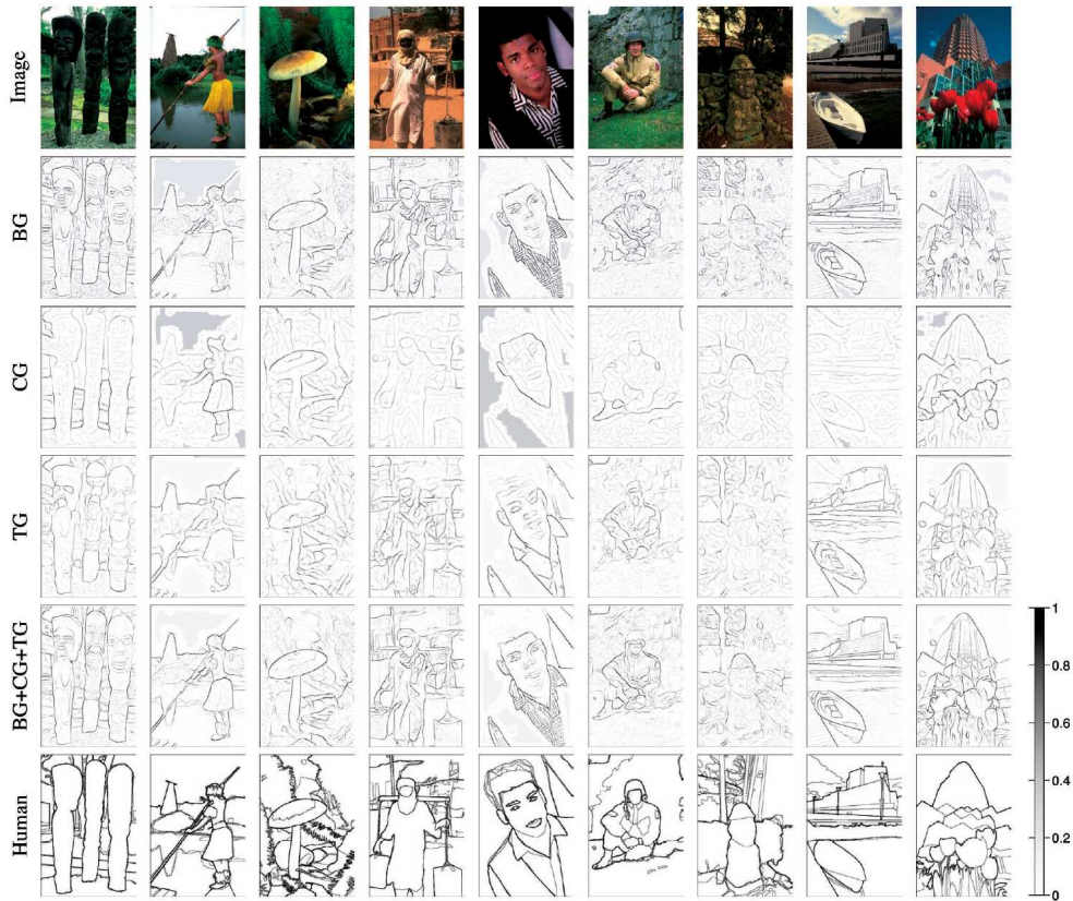
Figure 7.39 Combined brightness, color, texture boundary detector (Martin, Fowlkes, and Malik 2004) © 2004 IEEE. Successive rows show the outputs of the brightness gradient (BG), color gradient (CG), texture gradient (TG), and combined (BG+CG+TG) detectors. The final row shows human-labeled boundaries derived from a database of hand-segmented images (Martin, Fowlkes et al. 2001).
