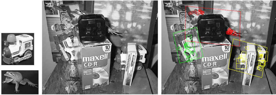
Figure 7.23 Recognizing objects in a cluttered scene (Lowe 2004) © 2004 Springer. Two of the training images in the database are shown on the left. These are matched to the cluttered scene in the middle using SIFT features, shown as small squares in the right image. The affine warp of each recognized database image onto the scene is shown as a larger parallelogram in the right image.
