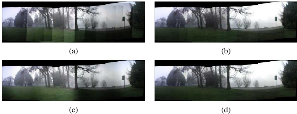
Figure 10.6 Simultaneous estimation of vignetting, exposure, and radiometric response (Goldman 2010) © 2011 IEEE: (a) original average of the input images; (b) after compensating for vignetting; (c) using gradient domain blending only (note the remaining mottled look); (d) after both vignetting compensation and blending.
