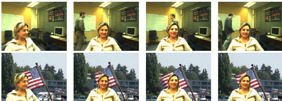
Figure 12.17 Background replacement using z-keying with a bi-layer segmentation algorithm (Kolmogorov, Criminisi et al. 2006) © 2006 IEEE.
