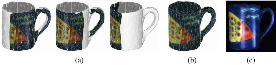
Figure 13.29 Estimating the diffuse albedo and reflectance parameters for a scanned 3D model (Sato, Wheeler, and Ikeuchi 1997) © 1997 ACM: (a) set of input images projected onto the model; (b) the complete diffuse reflection (albedo) model; (c) rendering from the reflectance model including the specular component.
