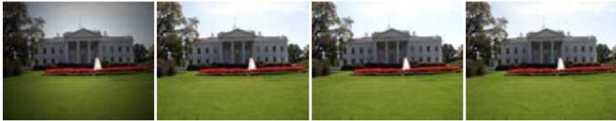
Figure 10.5 Single image vignetting correction (Zheng, Yu et al. 2008) © 2008 IEEE: (a) original image with strong visible vignetting; (b) vignetting compensation as described by Zheng, Zhou et al. (2006); (c–d) vignetting compensation as described by Zheng, Yu et al. (2008).
