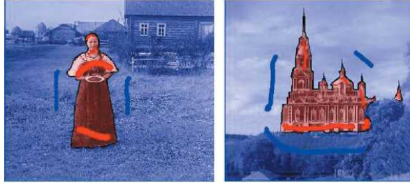
Figure 4.18 Image segmentation (Boykov and Funka-Lea 2006) © 2006 Springer: The user draws a few red strokes in the foreground object and a few blue ones in the background. The system computes color distributions for the foreground and background and solves a binary MRF. The smoothness weights are modulated by the intensity gradients (edges), which makes this a conditional random field (CRF).
