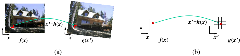
Figure 3.46 Forward warping algorithm: (a) a pixel f(x) is copied to its corresponding location x' = h(x) in image g(x') ; (b) detail of the source and destination pixel locations.
