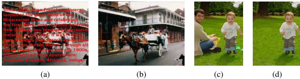
Figure 10.53 Image inpainting (hole filling): (a–b) propagation along isophote directions (Bertalmio, Sapiro et al. 2000) © 2000 ACM; (c–d) exemplar-based inpainting with confidence-based filling order (Criminisi, Pérez, and Toyama 2004).
