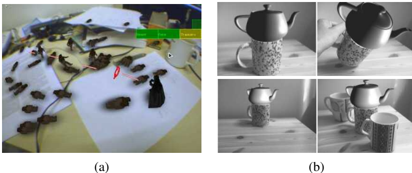
Figure 11.28 3D augmented reality: (a) Darth Vader and a horde of Ewoks battle it out on a table-top recovered using real-time, keyframe-based structure from motion (Klein and Murray 2007) © 2007 IEEE; (b) a virtual teapot is fixed to the top of a real-world coffee cup, whose pose is re-recognized at each time frame (Gordon and Lowe 2006) © 2007 Springer.
