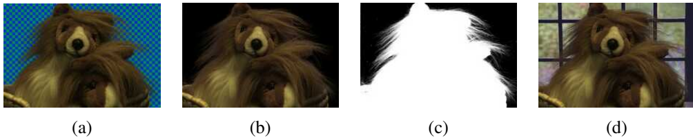
Figure 3.4 Image matting and compositing (Chuang, Curless et al. 2001) © 2001 IEEE: (a) source image; (b) extracted foreground object F ; (c) alpha matte \alpha shown in grayscale; (d) new composite C .
