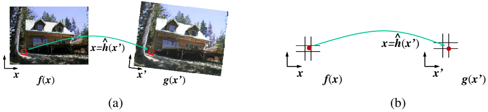
Figure 3.47 Inverse warping algorithm: (a) a pixel g(\mathbf{x}') is sampled from its corresponding location \mathbf{x} = \hat{\mathbf{h}}(\mathbf{x}') in image f(\mathbf{x}) ; (b) detail of the source and destination pixel locations.
