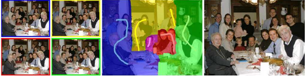
Figure 4.17 An unordered label MRF (Agarwala, Dontcheva et al. 2004) © 2004 ACM: Strokes in each of the source images on the left are used as constraints on an MRF optimization, which is solved using graph cuts. The resulting multi-valued label field is shown as a color overlay in the middle image, and the final composite is shown on the right.
