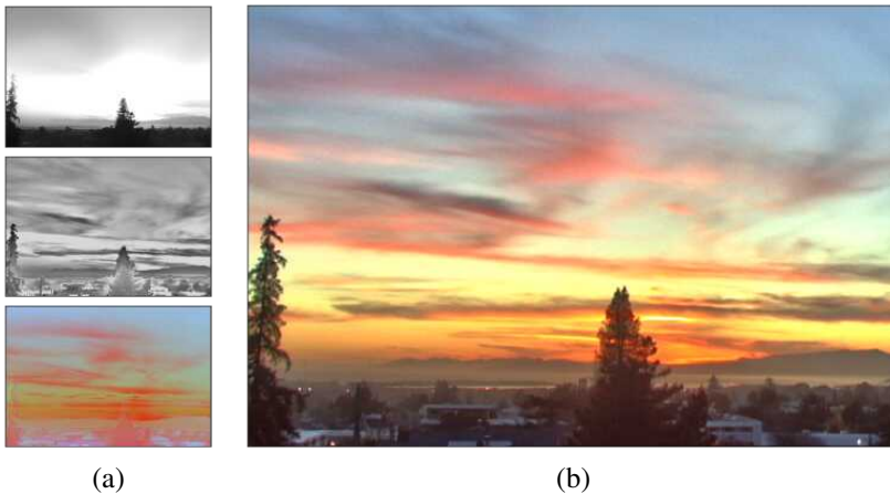
Figure 10.20 Local tone mapping using bilateral filter (Durand and Dorsey 2002): (a) low-pass and high-pass bilateral filtered log luminance images and color (chrominance) image; (b) resulting tone-mapped image (after attenuating the low-pass log luminance image) shows no halos. Processed images courtesy of Frédo Durand, MIT 6.815/6.865 course on Computational Photography.
