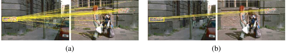
Figure 7.29 Matching based on visual words (Sivic and Zisserman 2009) © 2009 IEEE. (a) Features in the query region on the left are matched to corresponding features in a highly ranked video frame. (b) Results after removing the stop words and filtering the results using spatial consistency.
