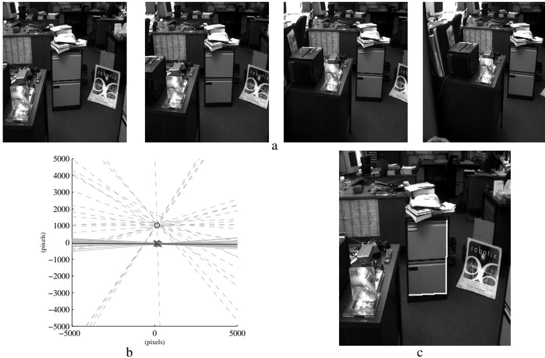
Fig. 19.6. **Planar motion sequence.** (a) Four images (of seven used) acquired from a camera mounted on a vehicle moving on a plane. (b) The computed epipoles ( $\times$ ), horizon lines (grey solid), and imaged screw axes (grey dashed) for all image pairs. (c) Euclidean invariants measured in the metric reconstruction the right angle is measured as  $89^\circ$ , the ratio of the non-parallel lengths is measured as 0.61 (compared to the approximate vertical value of 0.65).
