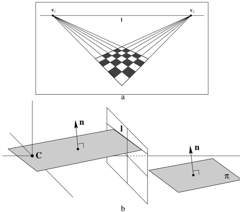
Fig. 8.16. **Vanishing line formation.** (a) The two sets of parallel lines on the scene plane converge to the vanishing points  $v_1$  and  $v_2$  in the image. The line  $l$  through  $v_1$  and  $v_2$  is the vanishing line of the plane. (b) The vanishing line  $l$  of a plane  $\pi$  is obtained by intersecting the image plane with a plane through the camera centre  $C$  and parallel to  $\pi$ .
