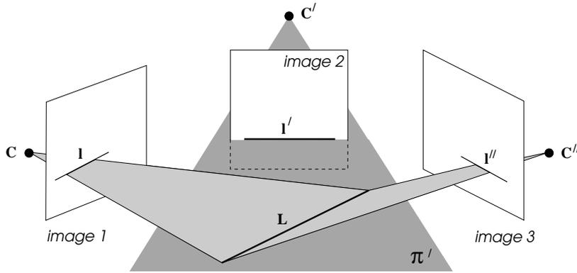
Fig. 15.3. **Line transfer.** The action on lines of the homography defined by figure 15.2 may similarly be visualized geometrically. A line,  $l$ , in the first image defines a plane in 3-space, which intersects  $\pi'$  in the line  $L$ . This line  $L$  is then imaged as the line  $l''$  in the third view.
