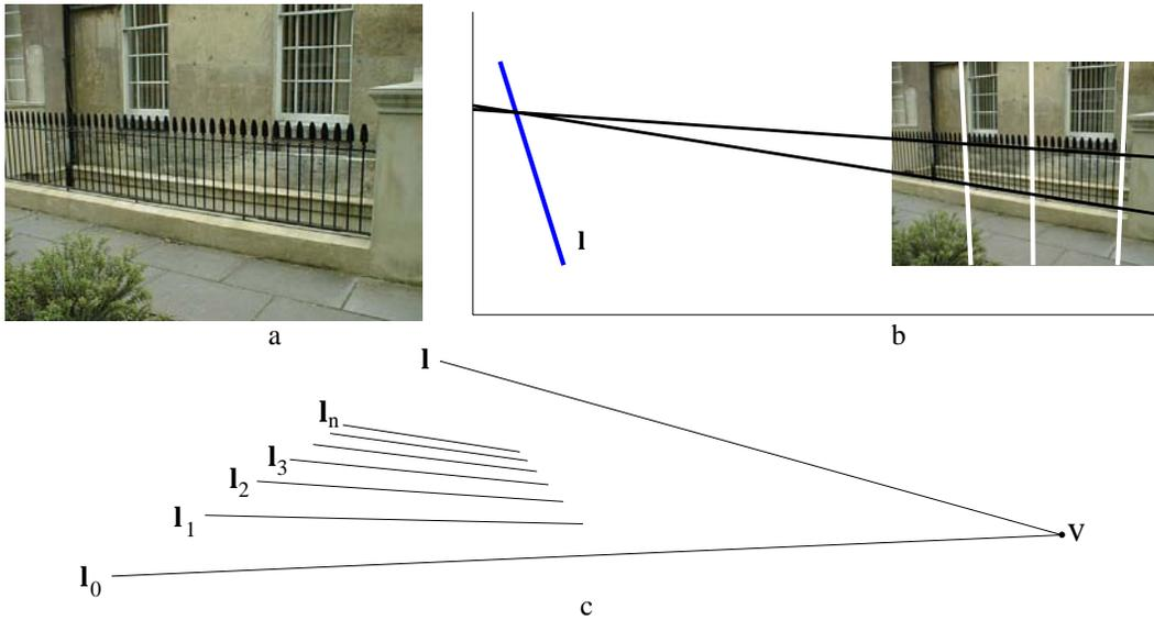
Fig. 8.18. **Determining a plane's vanishing line from imaged equally spaced parallel lines.** (a) Image of a vertical fence with equally spaced bars. (b) The computed vanishing line  $l$  from three equally spaced bars (12 apart). Note the vanishing point of the horizontal lines lies on this vanishing line. (c) The spacing between the imaged lines  $l_n$  monotonically decreases with  $n$ .
