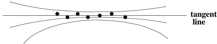
Fig. 11.7. Estimating a conic from point data (shown as  $\bullet$ ) may be poorly conditioned. All of the conics shown have residuals within the point error distribution. However, even though there is ambiguity in the estimated conic, the tangent line is well defined, and can be computed from the points.
