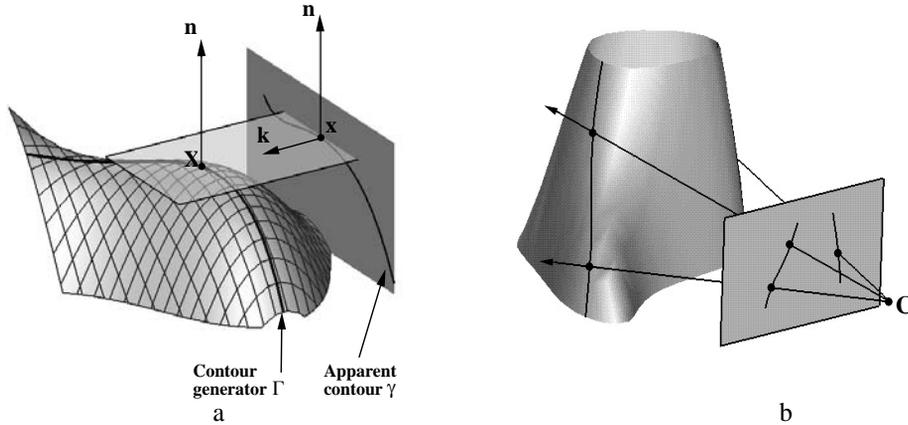
Fig. 8.3. **Contour generator and apparent contour.** (a) for parallel projection; (b) for central projection. The ray from the camera centre through  $\mathbf{x}$  is tangent to the surface at  $\mathbf{X}$ . The set of such tangent points  $\mathbf{X}$  defines the contour generator, and their image defines the apparent contour. In general the contour generator is a space curve. Figure courtesy of Roberto Cipolla and Peter Giblin.
