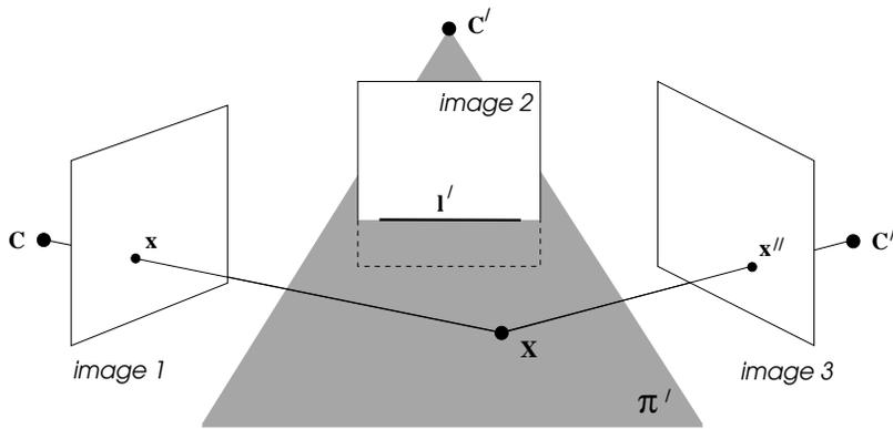
Fig. 15.2. **Point transfer.** A line  $l'$  in the second view back-projects to a plane  $\pi'$  in 3-space. A point  $x$  in the first image defines a ray in 3-space which intersects  $\pi'$  in the point  $X$ . This point  $X$  is then imaged as the point  $x''$  in the third view. Thus, any line  $l'$  induces a homography between the first and third views, defined by its back-projected plane  $\pi'$ .
