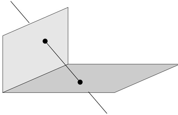
Fig. 3.1. A line may be specified by its points of intersection with two orthogonal planes. Each intersection point has 2 degrees of freedom, which demonstrates that a line in  $\mathbb{P}^3$  has a total of 4 degrees of freedom.
