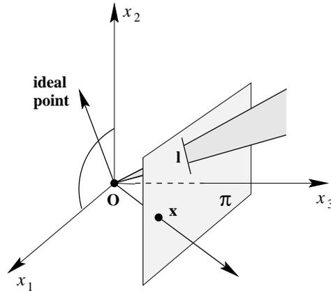
Fig. 2.1. **A model of the projective plane.** Points and lines of  $\mathbb{P}^2$  are represented by rays and planes, respectively, through the origin in  $\mathbb{R}^3$ . Lines lying in the  $x_1x_2$ -plane represent ideal points, and the  $x_1x_2$ -plane represents  $l_\infty$ .
