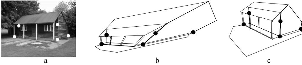
Fig. 10.6. **Direct reconstruction.** *The projective reconstruction of figure 10.3 may be upgraded to metric by specifying the position of five (or more) world points: (a) the five points used; (b) the corresponding points on the projective reconstruction of figure 10.3; (c) the reconstruction after the five points are mapped to their world positions.*
