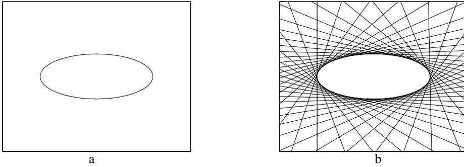
Fig. 2.2. (a) Points  $\mathbf{x}$  satisfying  $\mathbf{x}^T \mathbf{C} \mathbf{x} = 0$  lie on a point conic. (b) Lines  $\mathbf{l}$  satisfying  $\mathbf{l}^T \mathbf{C}^* \mathbf{l} = 0$  are tangent to the point conic  $\mathbf{C}$ . The conic  $\mathbf{C}$  is the envelope of the lines  $\mathbf{l}$ .
