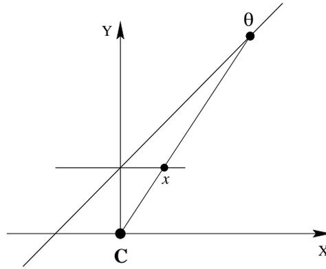
Fig. A3.1. The imaging setup for a simple estimation problem. A point on the line  $Y = X + 1$  is imaged by a line camera. The projection mapping is given by  $f : \theta \mapsto x = \theta/(1 + \theta)$ , where  $\theta$  parametrizes the points on the line  $Y = X + 1$ . Measurement is subject to noise with a zero-mode distribution.
