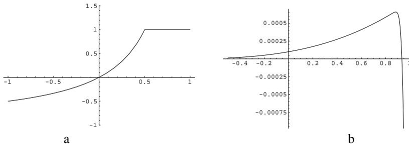
Fig. A3.4. (a) If the range of possible values of the world-point parameter  $\theta$  is limited to the range  $\theta \leq 1$ , then the ML estimate of any point  $x > 1/2$  will be  $\theta = 1$ . This will prevent infinite bias in the estimate, but there will still be bias. (b) The bias  $E_\theta[\hat{\theta}(x)] - \theta = \int_x \hat{\theta}(x)p(x|\theta)dx - \theta$  as a function of  $\theta$ . Measurement noise is Gaussian with  $\sigma = 0.01$ .
