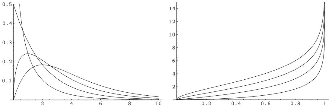
Fig. A2.1. The  $\chi_n^2$  distribution (left) and inverse cumulative  $\chi_n^2$  distribution  $F_n^{-1}$  (right) for  $n = 1, \dots, 4$ . In both cases, graphs are for  $n = 1, \dots, 4$  bottom to top (at middle point of horizontal axis).
