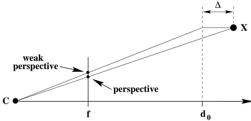
Fig. 6.8. **Perspective vs weak perspective projection.** The action of the weak perspective camera is equivalent to orthographic projection onto a plane (at  $Z = d_0$ ), followed by perspective projection from the plane. The difference between the perspective and weak perspective image point depends both on the distance  $\Delta$  of the point  $\mathbf{X}$  from the plane, and the distance of the point from the principal ray.
