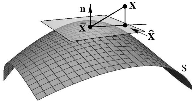
Fig. 5.2. Geometry of the errors in measurement space using the tangent plane approximation to  $S_M$ . The estimated point  $\hat{\mathbf{X}}$  is the closest point on  $S_M$  to the measured point  $\mathbf{X}$ . The residual error is the distance between the measured point  $\mathbf{X}$  and  $\hat{\mathbf{X}}$ . The estimation error is the distance from  $\hat{\mathbf{X}}$  to the true point  $\bar{\mathbf{X}}$ .
