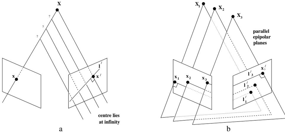
Fig. 14.1. **Affine epipolar geometry.** (a) Correspondence geometry: Projection rays are parallel and intersect at infinity. A point  $x$  back-projects to a ray in 3-space defined by the first camera centre (at infinity) and  $x$ . This ray is imaged as a line  $Y'$  in the second view. The 3-space point  $X$  which projects to  $x$  lies on this ray, so the image of  $X$  in the second view lies on  $Y'$ . (b) Epipolar lines and planes are parallel.
