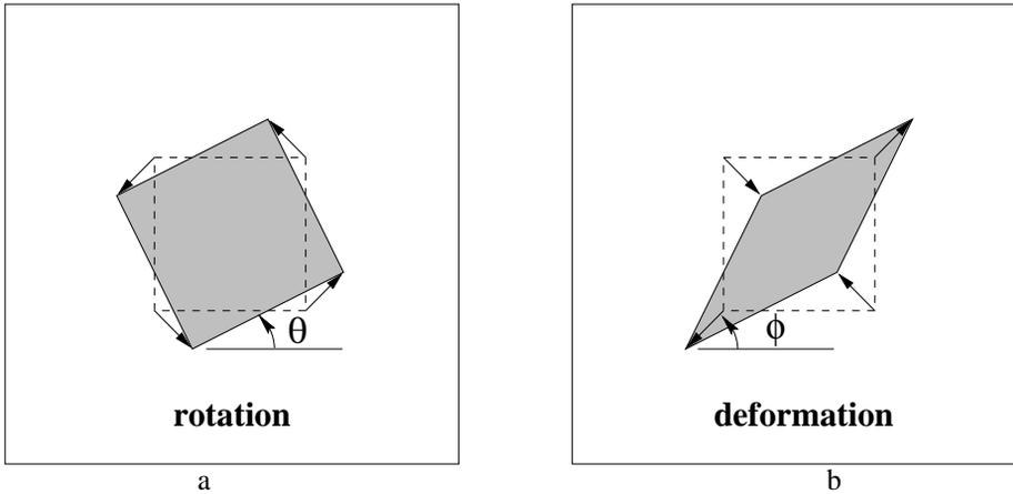
Fig. 2.7. **Distortions arising from a planar affine transformation.** (a) Rotation by  $R(\theta)$ . (b) A deformation  $R(-\phi)DR(\phi)$ . Note, the scaling directions in the deformation are orthogonal.
