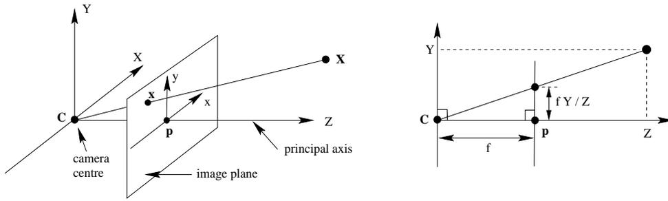
Fig. 6.1. **Pinhole camera geometry.**  $C$  is the camera centre and  $p$  the principal point. The camera centre is here placed at the coordinate origin. Note the image plane is placed in front of the camera centre.
