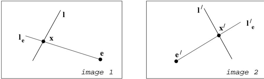
Fig. 13.5. The epipolar geometry induces a homography between corresponding lines  $l \leftrightarrow l'$  which are the images of a line  $L$  in 3-space. The points on  $l$  are mapped to points on  $l'$  as  $x' = [l']_{\times} Fx$ , where  $x$  and  $x'$  are the images of the intersection of  $L$  with the epipolar plane corresponding to  $l_e$  and  $l'_e$ .
