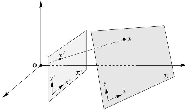
Fig. 2.3. **Central projection maps points on one plane to points on another plane.** The projection also maps lines to lines as may be seen by considering a plane through the projection centre which intersects with the two planes  $\pi$  and  $\pi'$ . Since lines are mapped to lines, central projection is a projectivity and may be represented by a linear mapping of homogeneous coordinates  $\mathbf{x}' = \mathbf{H}\mathbf{x}$ .
