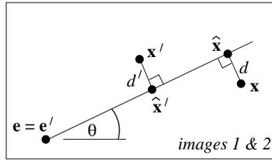
Fig. 12.9. **The epipolar geometry for pure translation.** In this case, corresponding epipolar lines are identical (see section 11.7.1(p293)). The epipolar line (parametrized by  $\theta$ ) that minimizes  $d^2 + d'^2$  can be computed directly.
