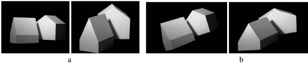
Fig. 11.11. **Image rectification.** (a) A pair of images of a house. (b) Resampled images computed from (a) using a projective transformation computed from  $F$ . Note, corresponding points in (b) match horizontally.
