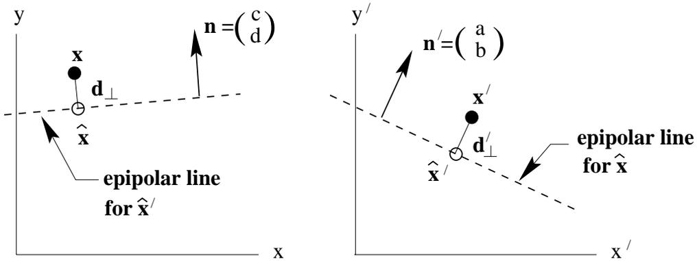
Fig. 14.3. The MLE of  $F_A$  from a set of measured corresponding points  $\{x_i \leftrightarrow x'_i\}$  involves estimating the five parameters  $a, b, c, d, e$  together with a set of correspondences  $\{\hat{x}_i \leftrightarrow \hat{x}'_i\}$  which exactly satisfy  $\hat{x}'_i{}^T F_A \hat{x}_i = 0$ . There is a linear solution to this problem.
