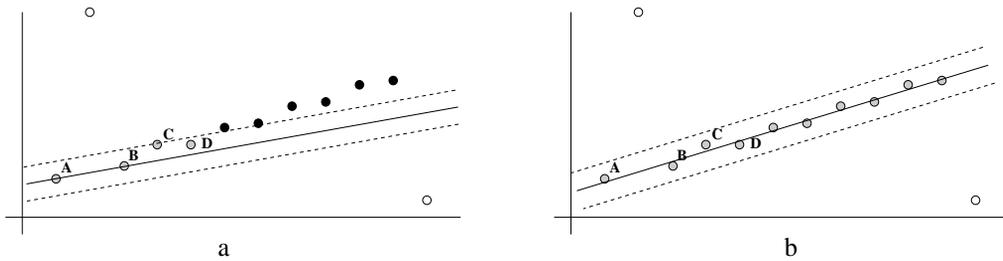
Fig. 4.8. **Robust ML estimation.** The grey points are classified as inliers to the line. (a) A line defined by points  $\langle \mathbf{A}, \mathbf{B} \rangle$  has a support of four (from points  $\{\mathbf{A}, \mathbf{B}, \mathbf{C}, \mathbf{D}\}$ ). (b) The ML line fit (orthogonal least-squares) to the four points. This is a much improved fit over that defined by  $\langle \mathbf{A}, \mathbf{B} \rangle$ . 10 points are classified as inliers.
