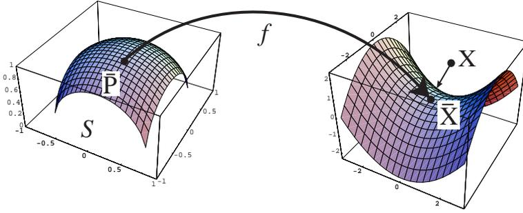
Fig. 5.4. **Back propagation (over-parametrized).** Mapping  $f$  maps constrained parameter surface to measurement space. A measurement  $\mathbf{X}$  is mapped (by a mapping  $\eta$ ) to the closest point on the surface  $f(S_P)$  and then back via  $f^{-1}$  to the parameter space, providing the ML estimate of the parameters. The covariance of  $\mathbf{X}$  is transferred via  $f^{-1} \circ \eta$  to a covariance of the parameters.
