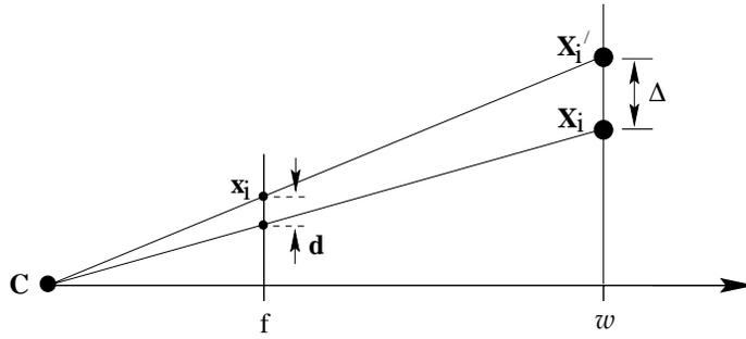
Fig. 7.2. The DLT algorithm minimizes the sum of squares of geometric distance  $\Delta$  between the point  $\mathbf{X}_i$  and the point  $\mathbf{X}_i'$  mapping exactly onto  $\mathbf{x}_i$  and lying in the plane through  $\mathbf{X}_i$  parallel to the principal plane of the camera. A short calculation shows that  $w\Delta = f\Delta$ .
