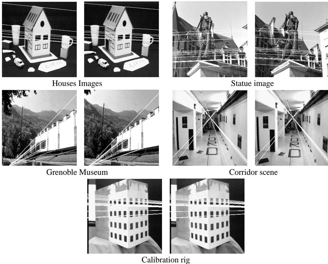
Fig. 11.2. Image pairs used for the algorithm comparison. In the top two the epipoles are far from the image centres. In the middle two the epipoles are close (Grenoble) and in the image (Corridor). For the calibration images the matched points are known extremely accurately.
