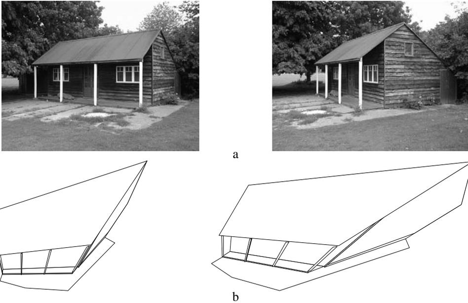
Fig. 10.3. **Projective reconstruction.** (a) Original image pair. (b) 2 views of a 3D projective reconstruction of the scene. The reconstruction requires no information about the camera matrices, or information about the scene geometry. The fundamental matrix  $F$  is computed from point correspondences between the images, camera matrices are retrieved from  $F$ , and then 3D points are computed by triangulation from the correspondences. The lines of the wireframe link the computed 3D points.
