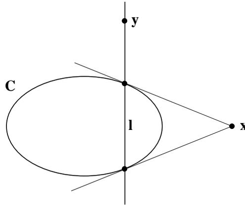
Fig. 2.19. **The pole–polar relationship.** The line  $l = Cx$  is the polar of the point  $x$  with respect to the conic  $C$ , and the point  $x = C^{-1}l$  is the pole of  $l$  with respect to  $C$ . The polar of  $x$  intersects the conic at the points of tangency of lines from  $x$ . If  $y$  is on  $l$  then  $y^T l = y^T Cx = 0$ . Points  $x$  and  $y$  which satisfy  $y^T Cx = 0$  are conjugate.
