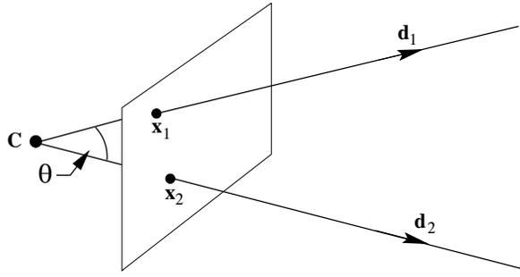
Fig. 8.11. The angle  $\theta$  between two rays.
