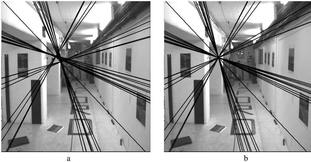
Fig. 11.1. **Epipolar lines.** (a) the effect of a non-singular fundamental matrix. Epipolar lines computed as  $l' = Fx$  for varying  $x$  do not meet in a common epipole. (b) the effect of enforcing singularity using the SVD method described here.
