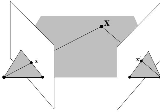
Fig. 10.1. **Triangulation.** The image points  $\mathbf{x}$  and  $\mathbf{x}'$  back project to rays. If the epipolar constraint  $\mathbf{x}'^T \mathbf{F} \mathbf{x} = 0$  is satisfied, then these two rays lie in a plane, and so intersect in a point  $\mathbf{X}$  in 3-space.
