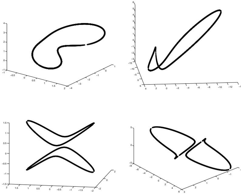
Fig. 22.8. Examples of elliptic quartic curves generated as the intersection of two ruled quadrics.
