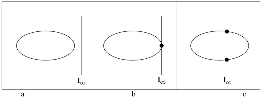
Fig. 2.20. **Affine classification of point conics.** A conic is an (a) ellipse, (b) parabola, or (c) hyperbola; according to whether it (a) has no real intersection, (b) is tangent to (2-point contact), or (c) has 2 real intersections with  $l_\infty$ . Under an affine transformation  $l_\infty$  is a fixed line, and intersections are preserved. Thus this classification is unaltered by an affinity.
