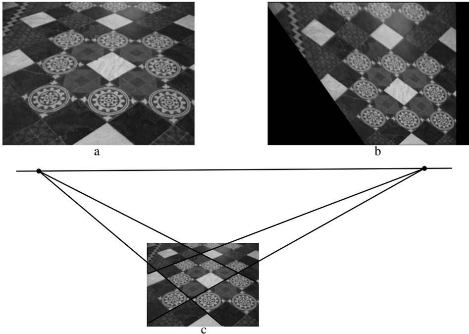
Fig. 2.13. **Affine rectification via the vanishing line.** The vanishing line of the plane imaged in (a) is computed (c) from the intersection of two sets of imaged parallel lines. The image is then projectively warped to produce the affinely rectified image (b). In the affinely rectified image parallel lines are now parallel. However, angles do not have their veridical world value since they are affinely distorted. See also figure 2.17.
