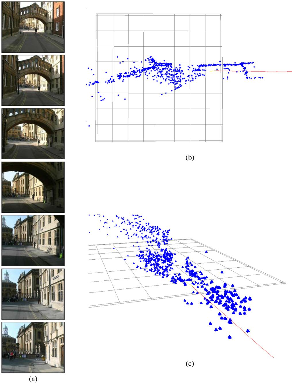
Fig. 1.3. **Reconstruction.** (a) Seven frames of a 700 frame sequence acquired by a hand held camera whilst walking down a street in Oxford. (b)(c) Two views of the reconstructed point cloud and camera path (the red curve). Figures courtesy of David Capel and 2d3 ([www.2d3.com](http://www.2d3.com)).
