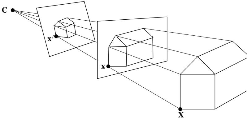
Fig. 8.5. **The cone of rays with vertex the camera centre.** An image is obtained by intersecting this cone with a plane. A ray between a 3-space point  $\mathbf{X}$  and the camera centre  $\mathbf{C}$  pierces the planes in the image points  $\mathbf{x}$  and  $\mathbf{x}'$ . All such image points are related by a planar homography,  $\mathbf{x}' = \mathbf{H}\mathbf{x}$ .
