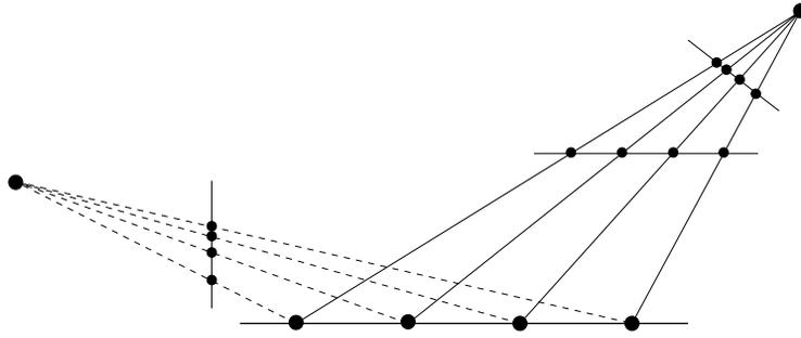
Fig. 2.8. **Projective transformations between lines.** There are four sets of four collinear points in this figure. Each set is related to the others by a line-to-line projectivity. Since the cross ratio is an invariant under a projectivity, the cross ratio has the same value for all the sets shown.
