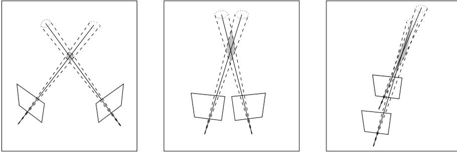
Fig. 12.6. **Uncertainty of reconstruction.** The shaded region in each case illustrates the shape of the uncertainty region, which depends on the angle between the rays. Points are less precisely localized along the ray as the rays become more parallel. Forward motion in particular can give poor reconstructions since rays are almost parallel for much of the field of view.
