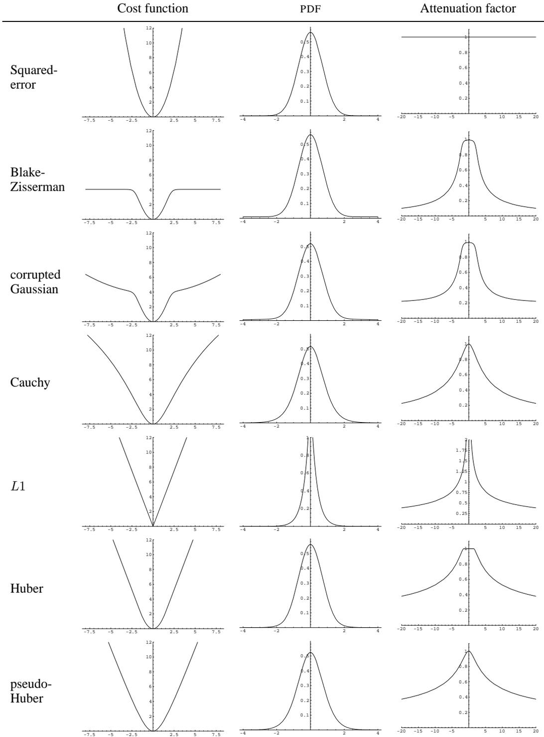
Fig. A6.4. A comparison of different cost functions,  $C(\delta)$ , for robust estimation. Their corresponding PDFs,  $\exp(-C(\delta))$ , and attenuation factors ( $w = C(\delta)^{1/2}/\delta$  see text) are also shown.
