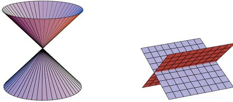
Fig. 3.4. **Degenerate quadrics.** The two most important degenerate quadrics are shown, the cone and two planes. Both these quadrics are ruled. The matrix representing the cone has rank 3, and the null-vector represents the nodal point of the cone. The matrix representing the two (non-coincident) planes has rank 2, and the two generators of the rank 2 null-space are two points on the intersection line of the planes.
