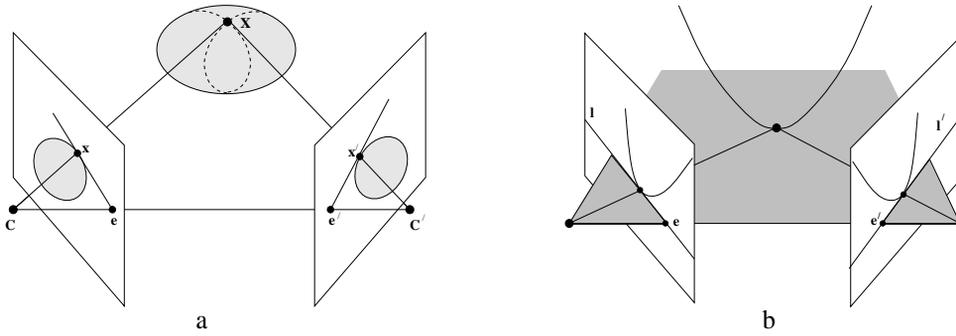
Fig. 11.6. **Epipolar tangency.** (a) for a surface; (b) for a space curve – figure after Porrill and Pollard [Porrill-91]. In (a) the epipolar plane  $CC'X$  is tangent to the surface at  $X$ . The imaged outline is tangent to the epipolar lines at  $x$  and  $x'$  in the two views. The dashed curves on the surface are the contour generators. In (b) the epipolar plane is tangent to the space curve. The corresponding epipolar lines  $l \leftrightarrow l'$  are tangent to the imaged curve.
