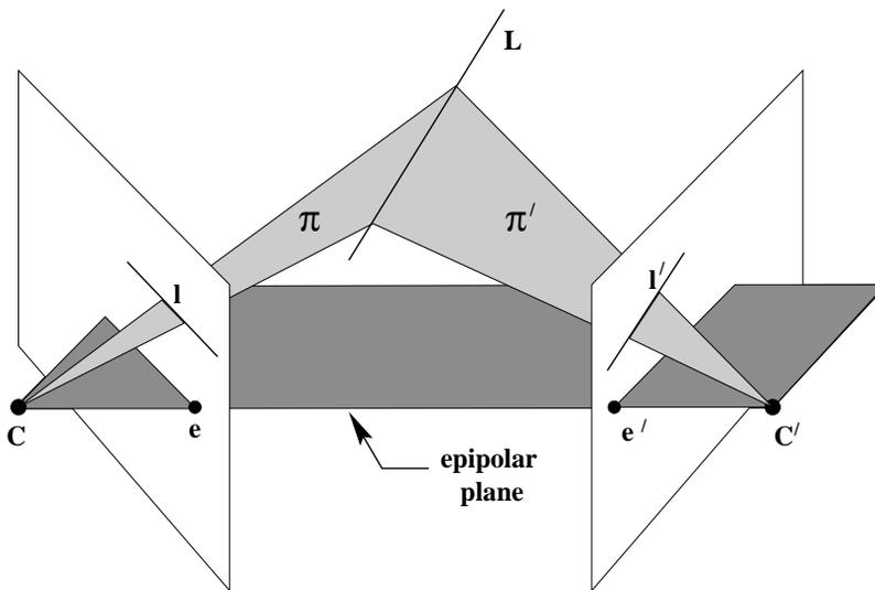
Fig. 12.8. **Line reconstruction.** The image lines  $l, l'$  back-project to planes  $\pi, \pi'$  respectively. The plane intersection determines the line  $L$  in 3-space. If the line in 3-space lies on an epipolar plane then its position in 3-space cannot be determined from its images. In this case the epipoles lie on the image lines.
