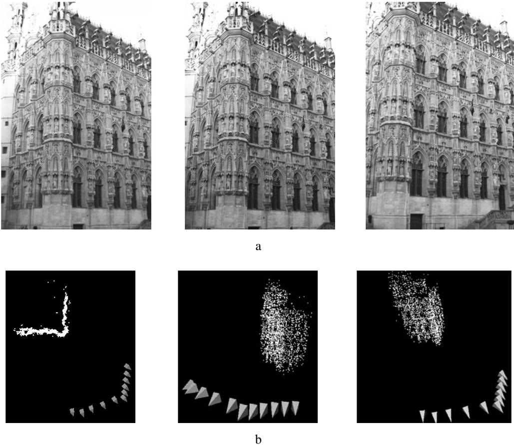
Fig. 1.5. (a) Three high resolution images ( $3000 \times 2000$  pixels) from a set of eleven of the cityhall in Leuven, Belgium. (b) Three views of a Euclidean reconstruction computed from the image set showing the 11 camera positions and point cloud.
