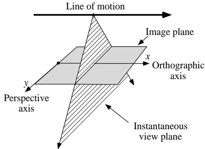
Fig. 6.9. Acquisition geometry of a pushbroom camera.
