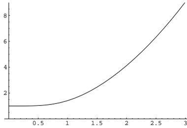
Fig. 5.5. RMS error in the position of a projected point  $\mathbf{x}'$  as a function of radial distance of  $\mathbf{x}'$  from the origin. The homography  $\mathbb{H}$  is computed from 4 evenly spaced points on a unit circle around the origin with errors in the second image only. The RMS error is proportional to the assumed error in the points used to compute  $\mathbb{H}$ , and the vertical axis is calibrated in terms of this assumed error.
