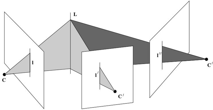
Fig. 15.1. A line  $L$  in 3-space is imaged as the corresponding triplet  $l \leftrightarrow l' \leftrightarrow l''$  in three views indicated by their centres,  $C, C', C''$ , and image planes. Conversely, corresponding lines back-projected from the first, second and third images all intersect in a single 3D line in space.
