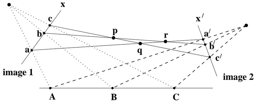
Fig. A7.4. **A line projectivity.** Points  $\{a, b, c\}$  are related to points  $\{A, B, C\}$  by a line-to-line perspectivity. Points  $\{a', b', c'\}$  are also related to points  $\{A, B, C\}$  by a perspectivity. However, points  $\{a, b, c\}$  are related to points  $\{a', b', c'\}$  by a projectivity; they are not related by a perspectivity because lines joining corresponding points are not concurrent. In fact the pairwise intersections result in three distinct points  $\{p, q, r\}$ .
