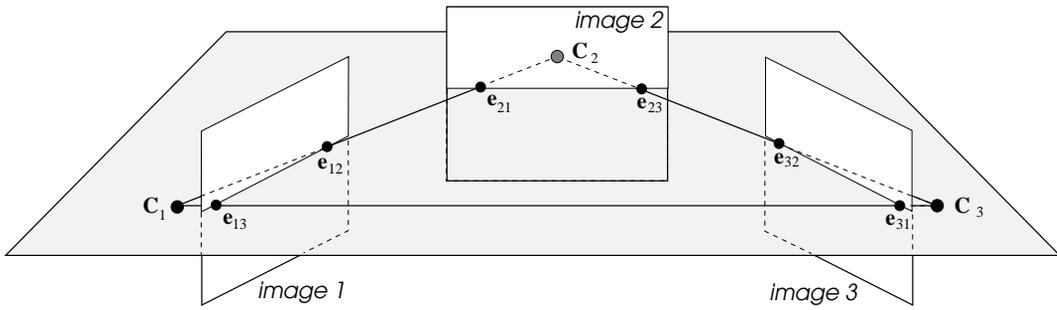
Fig. 15.8. **The trifocal plane** is defined by the three camera centres. The notation for the epipoles is  $e_{ij} = P_i C_j$ . Epipolar transfer fails for any point  $X$  on the trifocal plane. If the three camera centres are collinear then there is a one-parameter family of planes containing the three centres.
