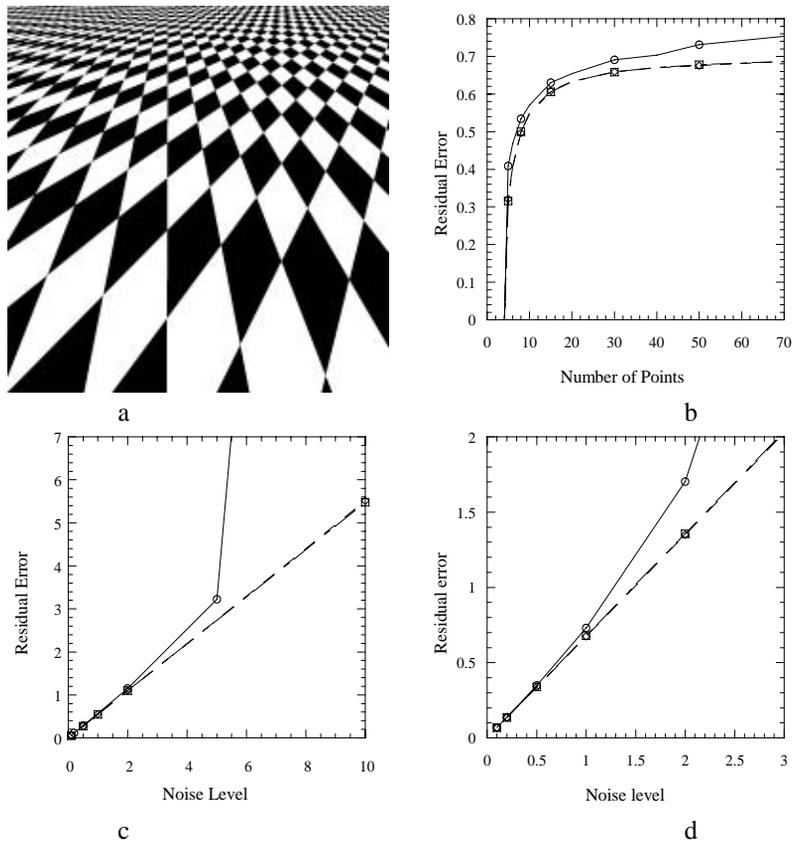
Fig. 4.6. **Comparison of the DLT and Gold Standard algorithms to the theoretical optimal residual error.** (a) The homography is computed between a chessboard and this image. In all three graphs, the result for the Gold Standard algorithm overlap and are indistinguishable from the theoretical minimum. (b) Residual error as a function of the number of points. (c) The effect of varying noise level for 10 points, and (d) 50 points.
