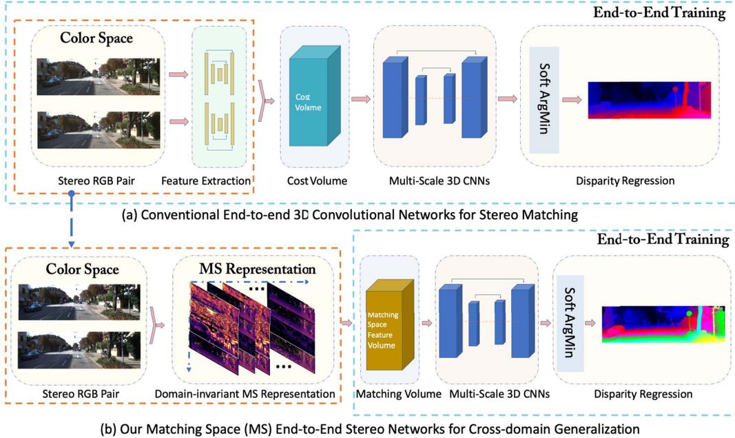
Figure 2: **Architecture overview.** (a) shows a conventional end-to-end 3D convolutional network for stereo matching. (b) illustrates our end-to-end MS-Nets architecture. The orange dashed boxes show the different feature extractors of the two architectures. The blue dashed boxes show the part of each network that is trained end-to-end. Feature extractors in MS-Nets are fixed and isolate the network from RGB.
