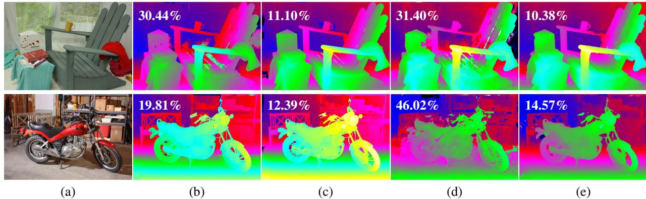
Figure 4: **Qualitative results on Middlebury 2014 [29] for networks trained on *sf-all*.** (a) Reference image, (b) to (e) disparity maps obtained with GCNet [17], MS-GCNet, PSMNet [5] and MS-PSMNet, respectively. Bad2-noc rates are superimposed on the disparities.
