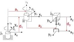
$$= \begin{bmatrix} -a_1 s_1 - a_2 s_{12} & -a_2 s_{12} & 0 \\ a_1 c_1 + a_2 c_{12} & a_2 c_{12} & 0 \\ 0 & 0 & -1 \end{bmatrix}$$
